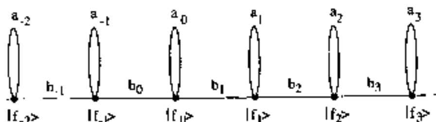
Fig. 10 Graphical representation of the most general tridiagonal Hamiltonian. The diagonal matrix elements are denoted by a_n ; the off-diagonal hopping integrals are denoted by b_n .
