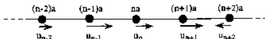
Fig. 1 Longitudinal displacements in a one-dimensional monatomic lattice. The equilibrium positions z_n = na are indicated by circles; the displacements u_n at a given instant are indicated by arrows.
